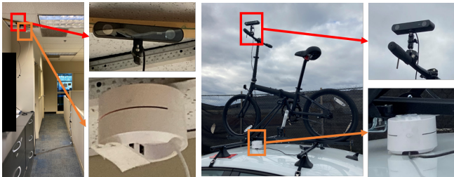
Fig. 3. Experiment Setup. In the Indoor setup, we mount a Google Nest WiFi AP and a StereoLabs ZED2 camera next to each other on the ceiling, while for outdoor setup, the camera is mounted on the handle of a roof-mounted bike. This setup simulates WiFi-enabled cameras that are becoming increasingly common.
